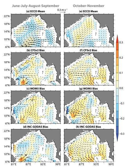
**FIGURE 5.** JJAS (a) mean ECCO2 surface currents (vectors, m s<sup>-1</sup>) and mean meridional current (shaded, m s<sup>-1</sup>), (b) bias in CFSv2 surface currents (vectors, m s<sup>-1</sup>) and mean meridional current (shaded, m s<sup>-1</sup>), (c) bias in MOM5, and (d) bias in INC-GODAS. (e–h) The same as (a–d) but for October-November (fall season).
