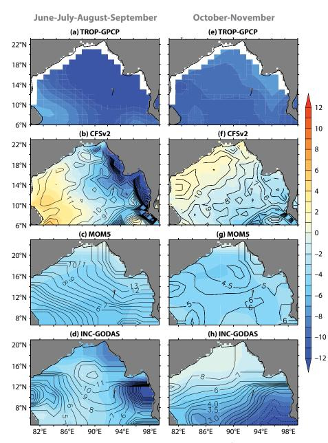
**FIGURE 4.** Evaporation minus precipitation (shaded; mm day<sup>-1</sup>) and bias (contours) during summer (June-July-August-September) for (a) TropFlux and Global Precipitation Climatology Project monthly precipitation (GPCP) data products, (b) CFSv2, (c) MOM5, and (d) INC-GODAS. (e–h) The same as (a–d) but for fall (October-November) season.
